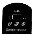
The D-Lux will start with its pre-set time setting of 10 sec ON and 30 sec OFF. The display will start counting down the ON time (10, 9, 8, etc.) and the SEC led will be flashing. When the ON time reaches 0 sec it will jump to the OFF time and starts counting down the OFF time (30, 29, etc.)
